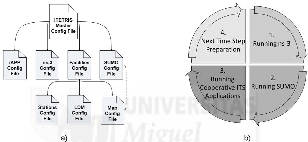
Figure 4-8. iTETRIS' configuration files hierarchy (a) and run-time loop iteration (b).
