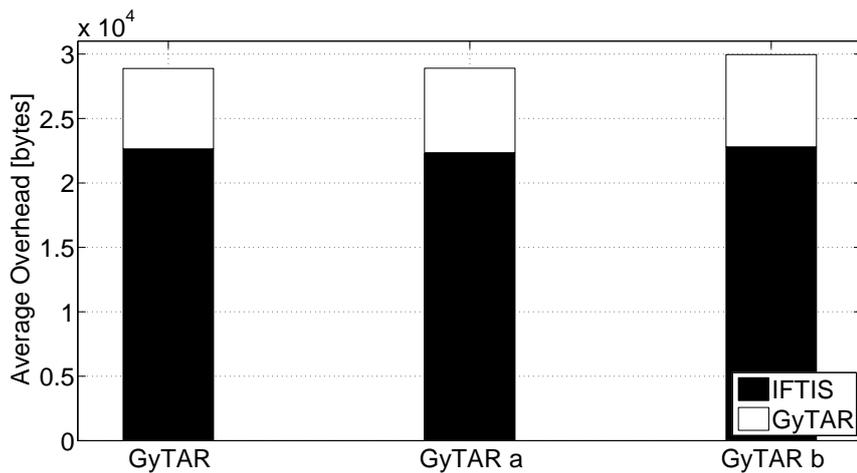
Figure 6-11. GyTAR’s average overhead for different variants of the adopted sender-based forwarding scheme.
