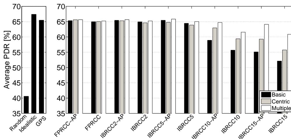
Figure 7-30. Average PDR of the basic injection strategies compared with that obtained using the centric and multiple injection strategy variants (5 injected messages; traffic Scenario 2).
