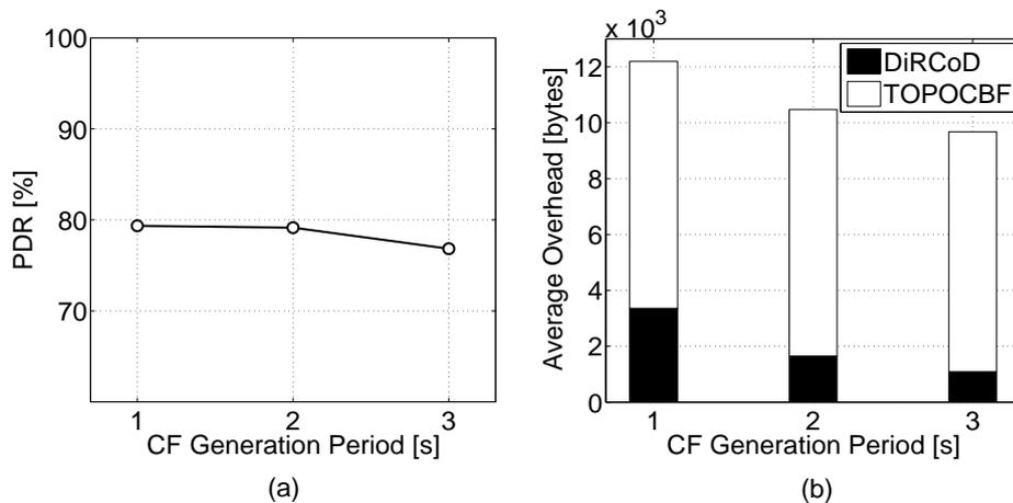
Figure 6-8. TOPOCBF's PDR (a) and average communications overhead (b) as a function of the DiRCoD *CF generation period* (30m  $R$ ; (*CF generation period*+0.5s) *CET*).
