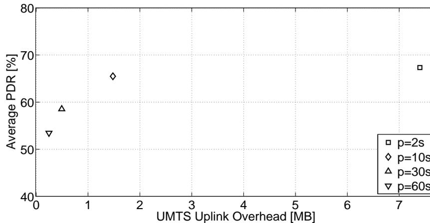
Figure 7-26. Average PDR as a function of the UMTS uplink overhead for various values of the GPS uploading period  $p$  (5 injected messages; traffic Scenario 2).
