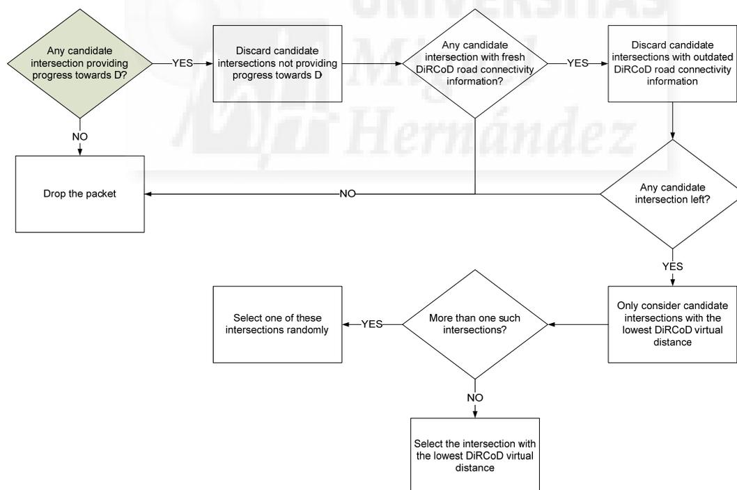
Figure 6-4. Flow diagram used for the TOPOCBF selection of target intersections.
