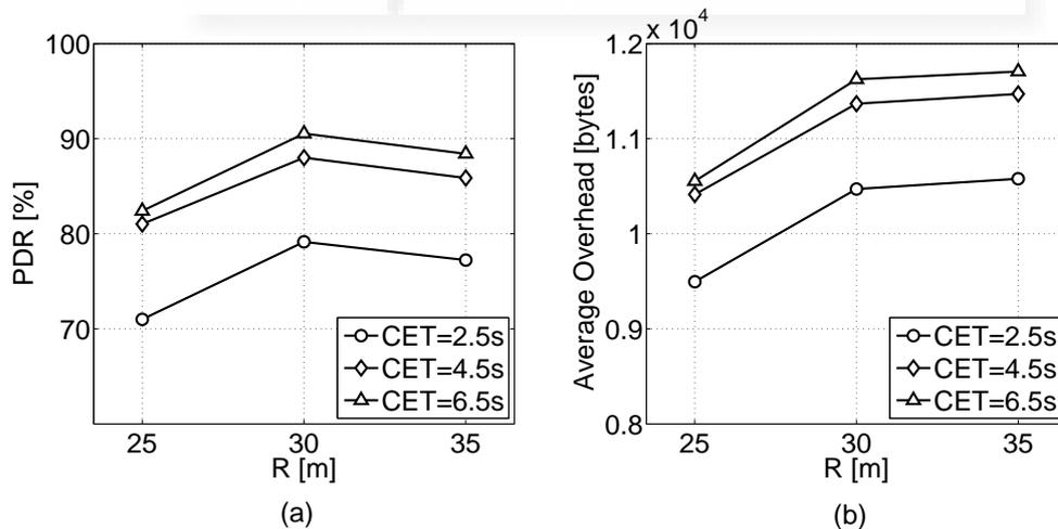
Figure 6-9. TOPOCBF's PDR (a) and average communications overhead (b) for varying values of  $R$  and  $CET$  (2s *CF generation period*).
