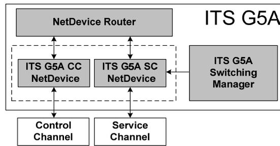
Figure 4-13. iTETRIS' ITS G5A communication module.
