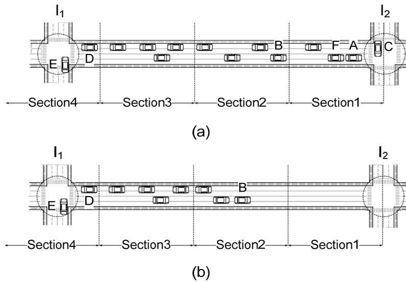
Figure 5-2. Road segment with DiRCoD full multi-hop connectivity (a), and DiRCoD partial multi-hop connectivity (b).
