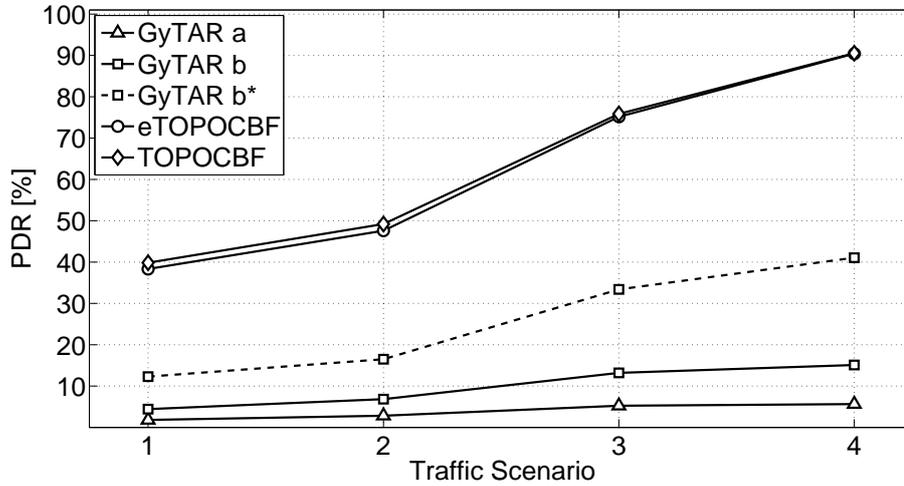
Figure 6-12. PDR for the four simulated traffic scenarios (23dBm transmission power).
