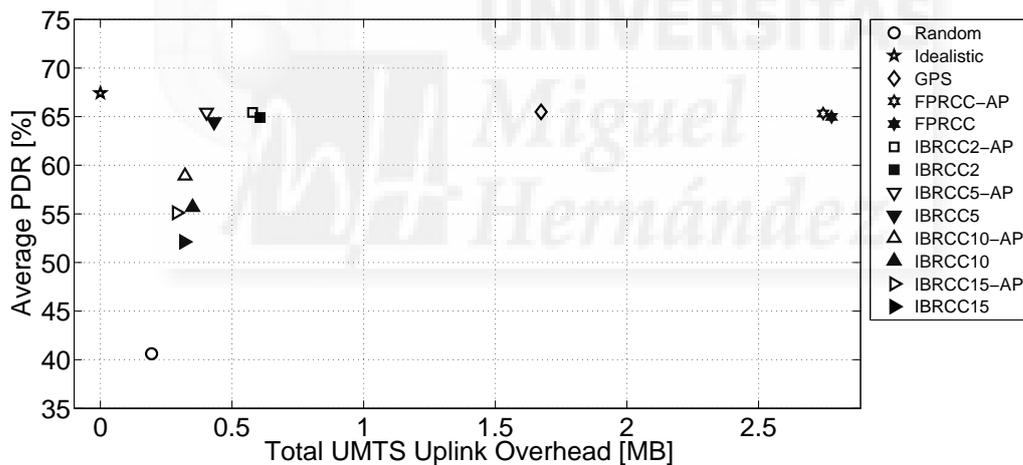
Figure 7-29. Average PDR vs. total communications overhead on the UMTS uplink channel (5 injected messages; traffic Scenario 2).
