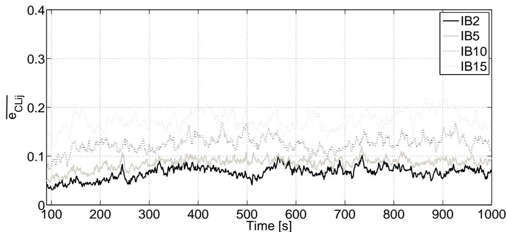
Figure 7-21. Time variation of the CL estimation error averaged over all the road segments of the road network (traffic Scenario 2).
