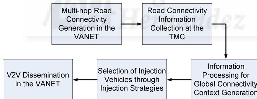
Figure 7-6. Flow diagram of RoAHD’s operation.
