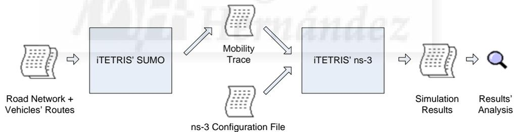
Figure 4-9. Simulation process with the ns-3 testbed.
