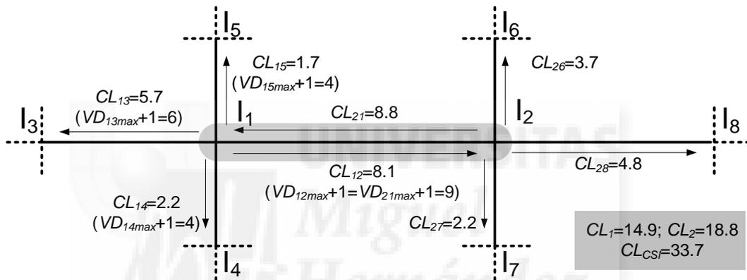
Figure 7-10. Example of CL computation for a connected set of intersections.
