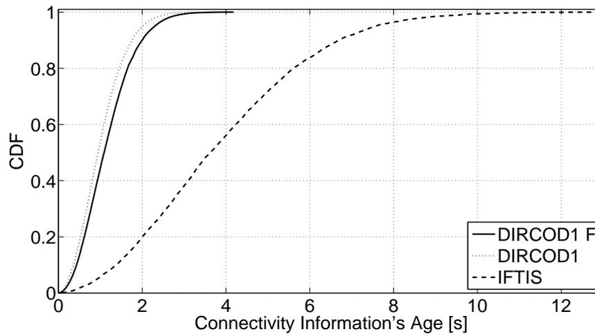
Figure 5-13. CDF of the connectivity information age at  $I_1$  (23dBm transmission tower, 10 vehicles/km/lane vehicular density).
