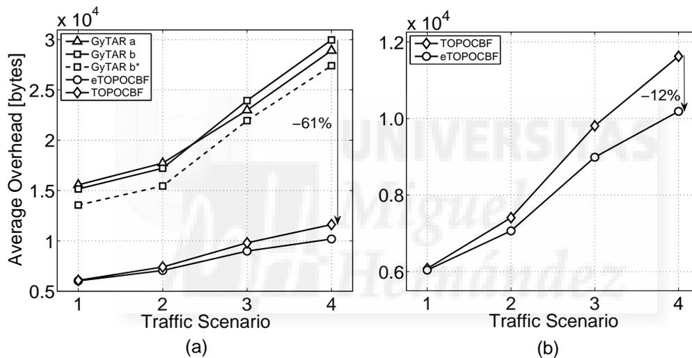
Figure 6-15. Average communications overhead for the four simulated traffic scenarios (23dBm transmission power).
