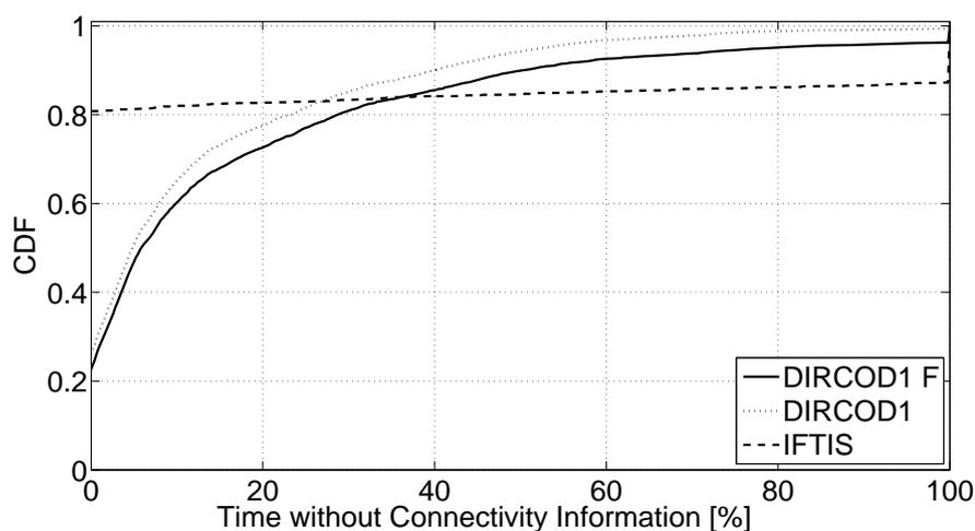
Figure 5-12. CDF of the percentage of time spent at  $I_1$  before receiving a connectivity estimate (23dBm transmission power, 10 vehicles/km/lane vehicular density).
