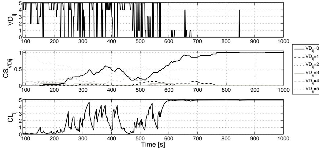
Figure 7-9. Example of CL computation for a road segment  $I_i \rightarrow I_j$ .
