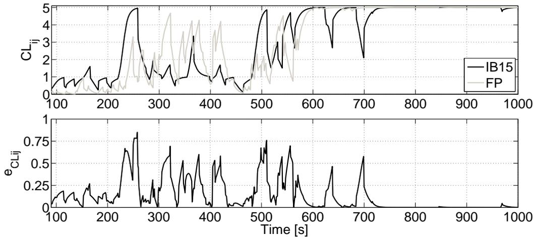
Figure 7-20. Time variation of the CL estimation error over a road segment  $I_i \rightarrow I_j$  (IB with  $T_U=15s$ ; traffic Scenario 2).
