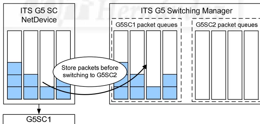
Figure 4-15. ITS G5 Switching manager operation.
