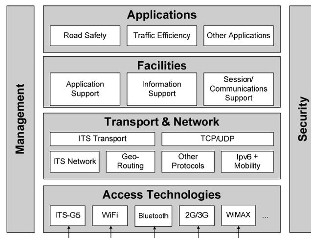
Figure 2-1. ETSI ITS Architecture for Intelligent Transport Systems Communications [28].
