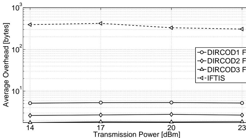
Figure 5-15. Additional communications overhead as a function of the transmission power (10 vehicles/km/lane vehicular density).
