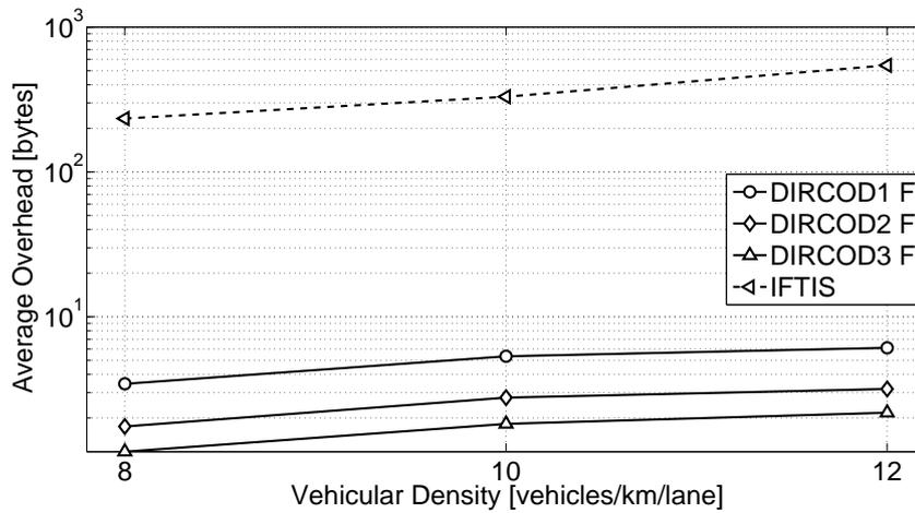
Figure 5-14. Additional communications overhead as a function of the vehicular density (20dBm transmission power).
