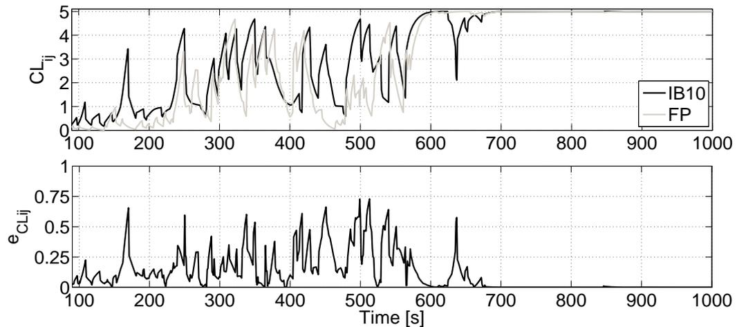
Figure 7-19. Time variation of the CL estimation error over a road segment  $I_i \rightarrow I_j$  (IB with  $T_U=10s$ ; traffic Scenario 2).
