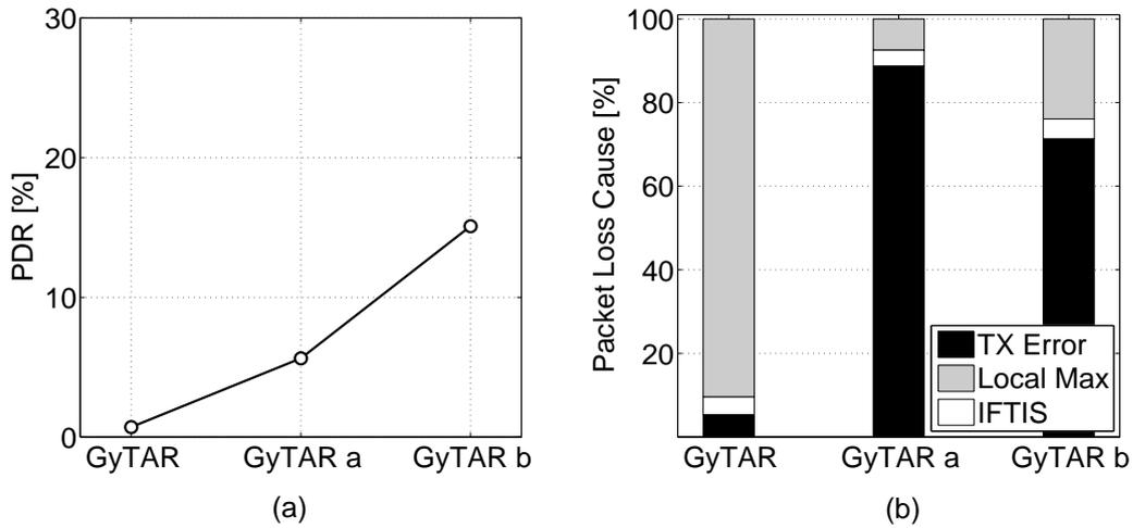
Figure 6-10. GyTAR’s PDR (a) and packet loss cause (b) for different variants of the adopted sender-based forwarding scheme.
