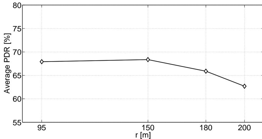
Figure 7-25. Average PDR as a function of the inter-vehicular distance  $r$  used for the computation of CSVs (5 injected messages; traffic Scenario 2).
