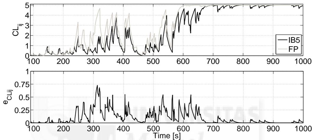
Figure 7-18. Time variation of the CL estimation error over a road segment  $I_i \rightarrow I_j$  (IB with  $T_U=5s$ ; traffic Scenario 2).
