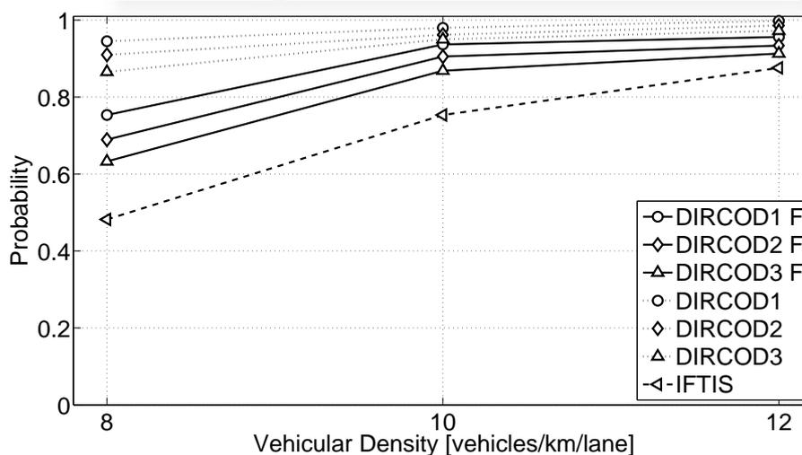
Figure 5-10. Connectivity information reception probability as a function of the vehicular density (20dBm transmission power).
