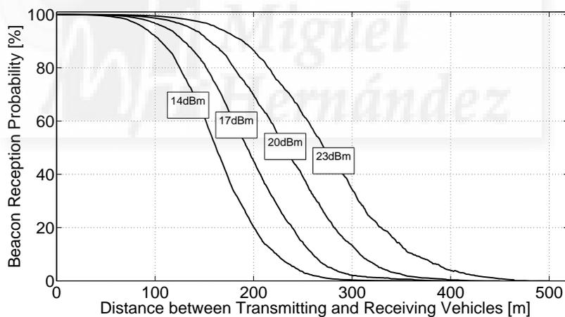
Figure 5-9. Beacon reception probability as a function of the distance between transmitting and receiving vehicles for different transmission powers.
