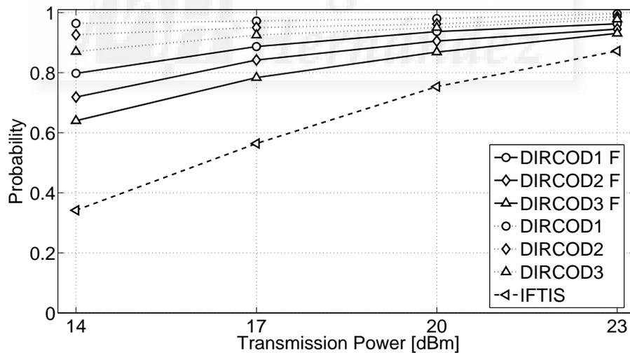
Figure 5-11. Connectivity information reception probability as a function of the transmission power (10 vehicles/km/lane vehicular density).
