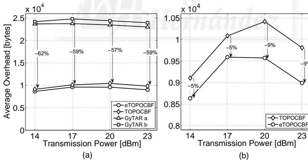
Figure 6-18. Average communications overhead as a function of the transmission power (traffic Scenario 3).
