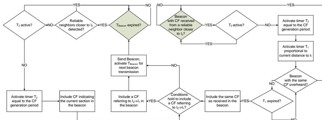
Figure 5-6. Flow diagram for the generation and forwarding of DiRCoD's  $CF$ s (direction  $I_1 \rightarrow I_2$ ).
