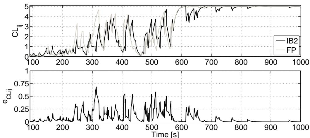
Figure 7-17. Time variation of the CL estimation error over a road segment  $I_i \rightarrow I_j$  (IB with  $T_U=2s$ ; traffic Scenario 2).
