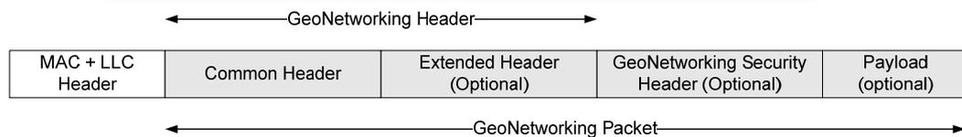
Figure 2-8. GeoNetworking packet structure.
