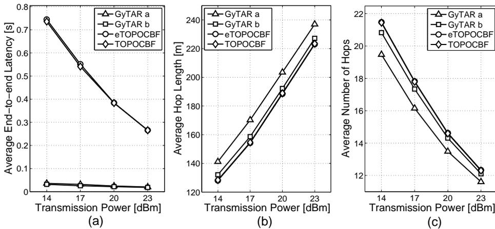
Figure 6-19. Average end-to-end latency (a), hop length (b), and number of hops (c) as a function of the transmission power (traffic scenario 3).
