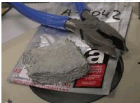
Figura 3. 6. Material no friable. Fibrocemento.[7]
