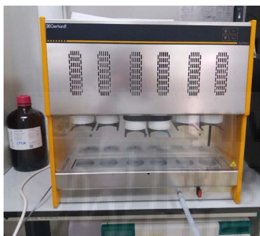
Figura 17. Extractor Soxhlet J.O, Selecta Mo.6003286.
