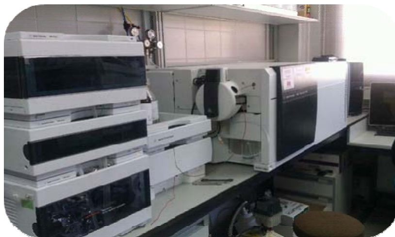
Picture 7.8. UHPLC coupled with a 6460 triple quadrupole-MS/MS (Agilent Technologies, Waldbronn, Germany)
