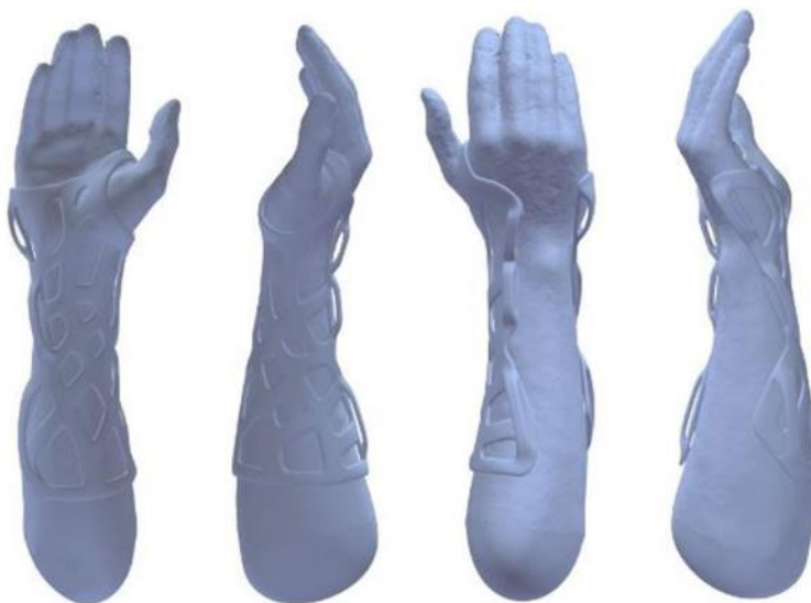
Fig. 3. A forearm cast is designed with the maximal possible number of openings compatible with adequate stability. Designing of the forearm cast based on the virtual forearm model is semi-automated. After completion it is translated into an STA (stereolithography) file.
