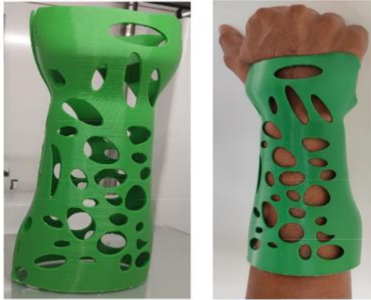
Fig. 6. (a) The image of the model after being printed. Fig. 6(b) Image of the cast worn on hand.
