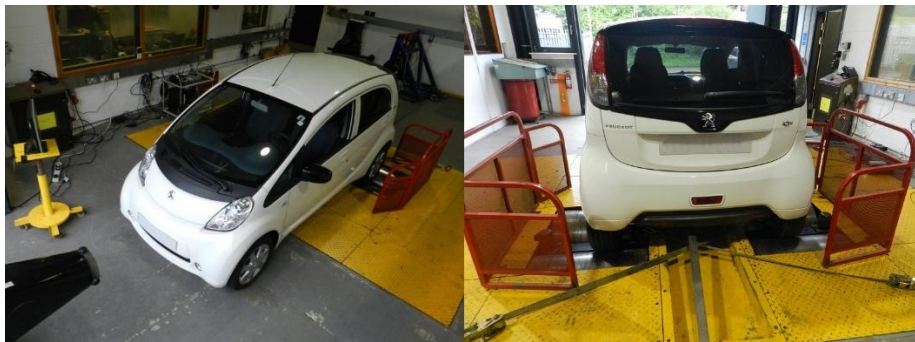
Fig. 10. Car installed on the roller bench
