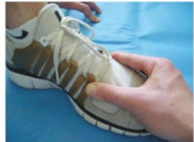
Straw method of measuring footwear length (B)
