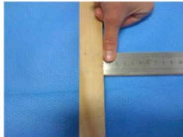
Straw method of measuring footwear length (A)
