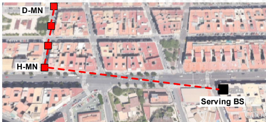
c) The H-MN reaches the intersection corner and experiences NLOS conditions with the BS
