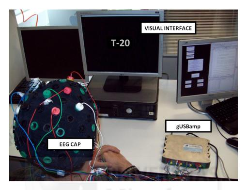
Figure 3.9: Real-time Brain-Machine Interface environment.
