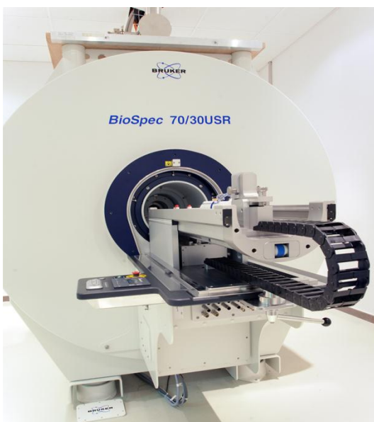
Figure 6: 7 Tesla magnet used in functional Magnetic Resonance Imaging experiments.
