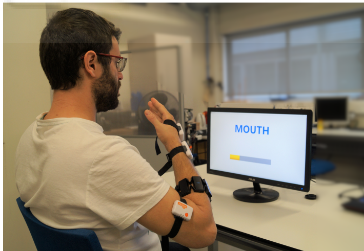
Figure 5.1: Experimental setup. The subjects wore three magneto-inertial devices placed onto the upper limb. Furthermore, the experts subjects performed the gestures with an sEMG armband. They were sat down in front of a screen where the desired gesture was shown.
