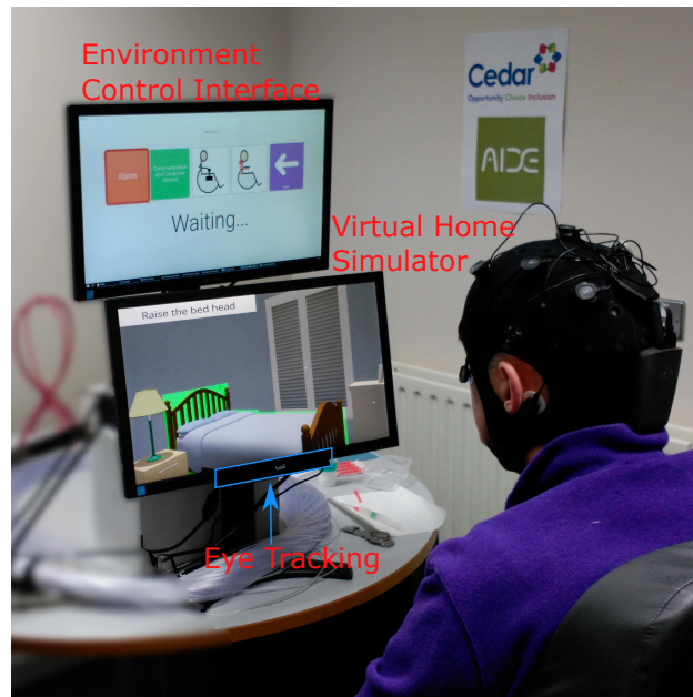
Figure 5.9: The experimental setup was composed by two screens: the ECI and the virtual environment. An eye tracking was placed in the virtual environment screen to detect the gaze point.
