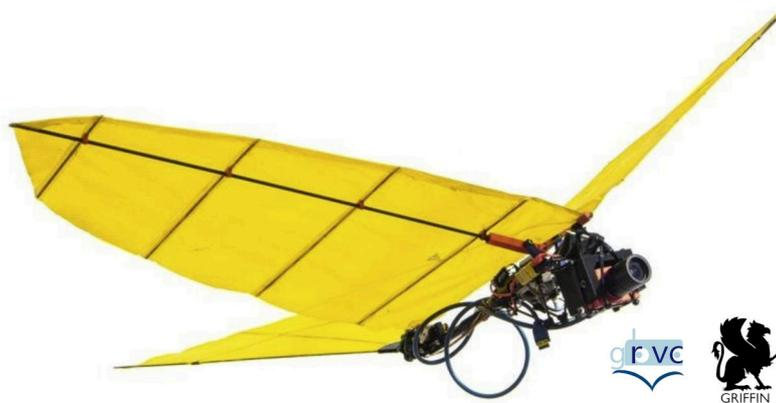
**Figure 1.2** GRIFFIN ornithopter prototype with an onboard DAVIS346 event camera. Adapted from [28].
