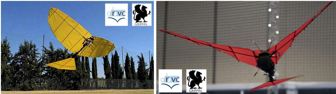
**Figure 1.1** GRIFFIN ornithopter prototypes designs by GRVC Robotics Laboratory of the University of Seville.
