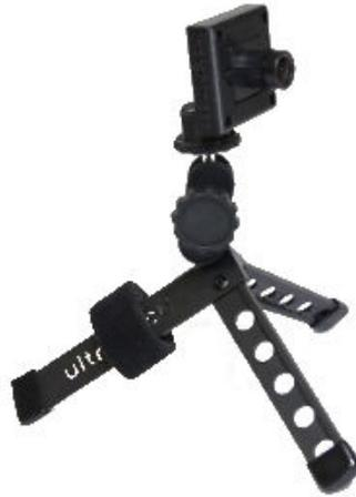
**Figure 2.27** Insightness Rino 3 Silicon Eye. Extracted from [30].
