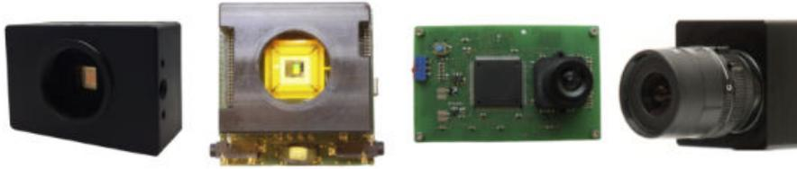
**Figure 2.24** Left to right. DVS240, DAVIS240, eDVS, DVS128. Adapted from [29].
