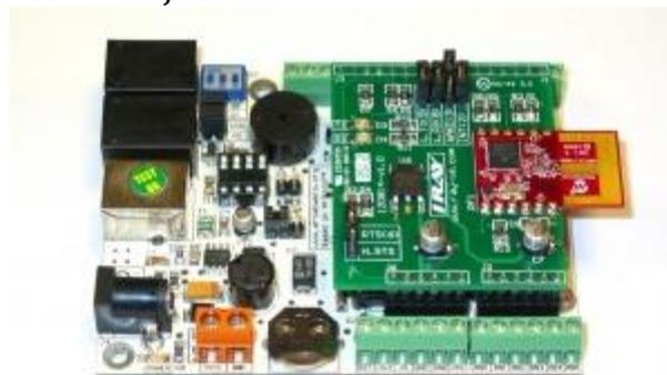
**Figura 54: Shield for Arduino MRF24J40MA**
