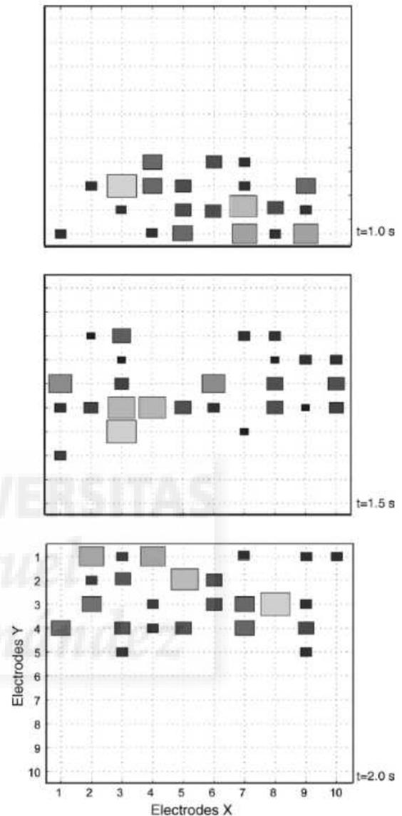
Fig. 4. Example of the animated frame by frame visualization. A sequence of three frames show the response to an upwardly moving bar at different times. Size and colour brightness represent the observed firing rate at a particular electrode location in the array.
