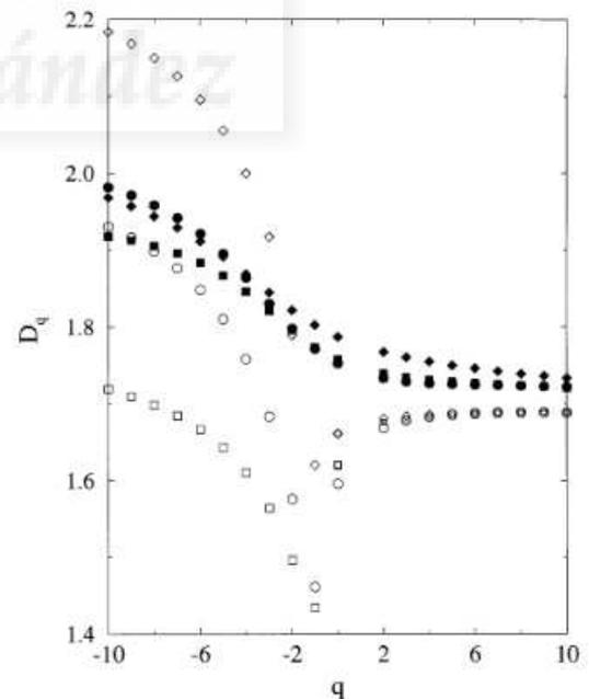
Fig. 5. Dependence of the generalised dimensions  $D_q$  on  $q$  for three diffusion-limited aggregation (DLA) clusters (circles, squares and diamonds) grown on a triangular lattice and having around 100 000 particles each. The results were obtained by using either the box-counting (empty symbols) or a generalised sand-box (filled symbols) method (see text).
