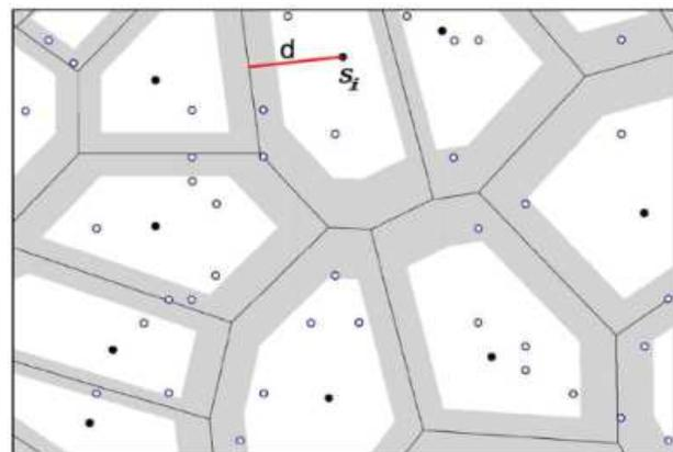
**Fig. 1.** Part of a Voronoi diagram (black lines) for a set of sites (filled circles). Bands around the edges of the Voronoi diagram are shown in grey. In this particular case  $\delta = 0.29$ , indicating the 29% of the distance  $d$  between a Voronoi edge and its closest site  $s_i$ . The  $P$  population is shown in open circles.
