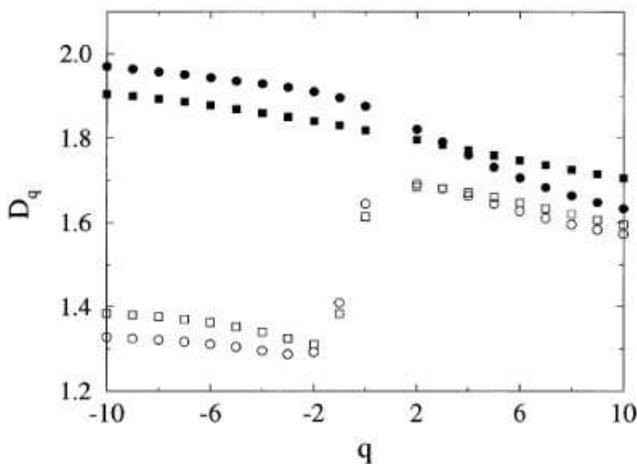
Fig. 3. Dependence of the generalised dimensions  $D_q$  on  $q$  for two neuronal cells of the turtle retina (circles and squares). The results were obtained by using either the box-counting (empty symbols) or a generalised sand-box (filled symbols) method (see text). The digitalised pictures of the cells contained around 20 000 pixels.
