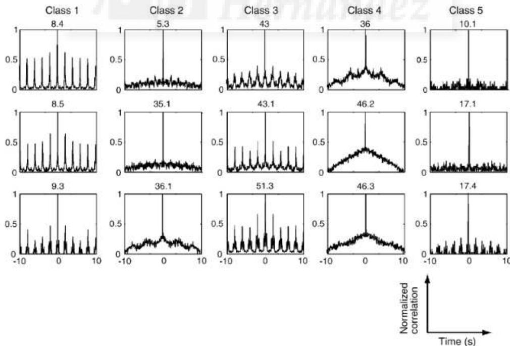
Fig. 5. Classification block. Each column shows a set of units according to the output of the clustering method. In this case, the relatives consisted of autocorrelated units (bin size: 50 ms and lag max: 200) clustered into five different classes. For simplicity, only three units belonging to each class are shown. Class numbers are indicated on top of each column. Unit identifiers are represented as the legends on top of the autocorrelograms panels.
