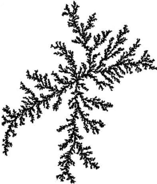
Fig. 2. Typical diffusion-limited aggregation (DLA) cluster containing around 100 000 particles generated on a triangular lattice.
