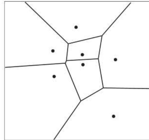
Fig. 2. Voronoi diagram (black lines) for a set of sites (filled circles). The polygons close to the borders of the sampling window remain open since there are no neighboring points in those directions.
