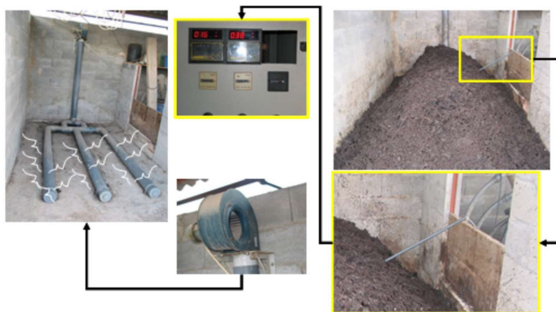
Figure 5.5. Detail of the Rutgers static pile system for composting.
