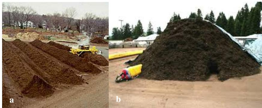
**Figure 10** – a: Windrow composting pile system (Adapted from [www.caerphilly.gov.uk/hovwp/en/organic\\_project.html](http://www.caerphilly.gov.uk/hovwp/en/organic_project.html)); B: aerated static pile composting system (Adapted from [www.compostsystems.com/](http://www.compostsystems.com/)).
