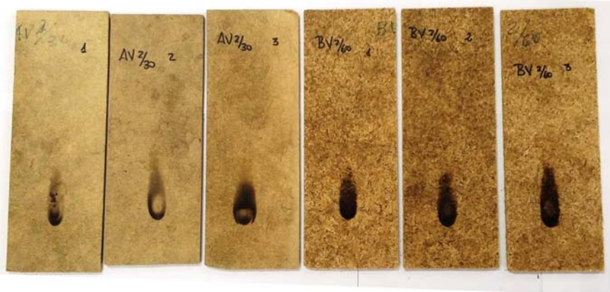
Fig 3. Samples after the fire reaction test.
