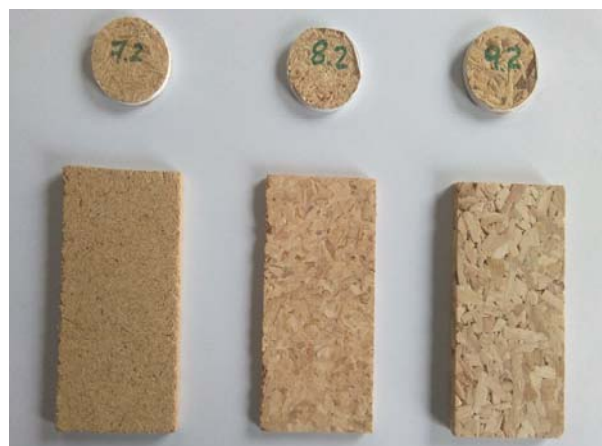
Fig 2. Acoustic and bending tests samples (circular and rectangular shape respectively) of the three types of panels.
