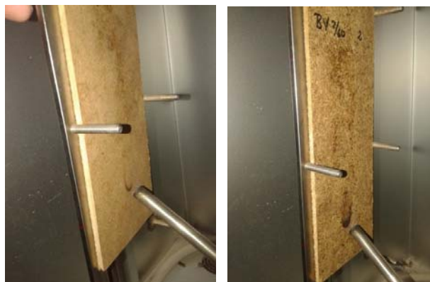
Fig 2. Specimens placed in the frame for reaction to fire test.
