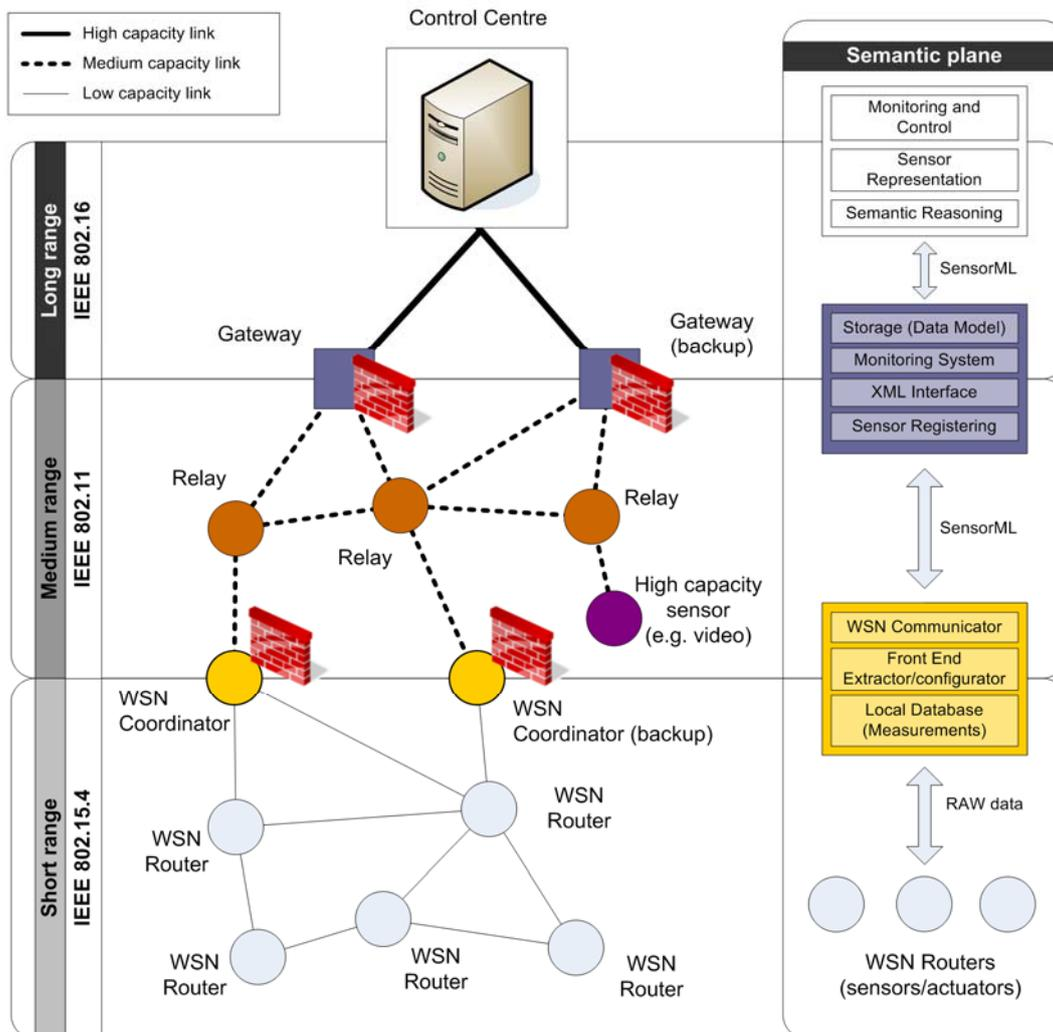
Fig. 1. FASyS's heterogeneous wireless communications architecture.
