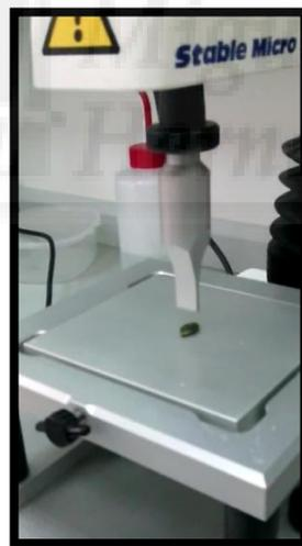
**Figura 24.** Sonda *Volodkevich bite jaws HDP/VB*
