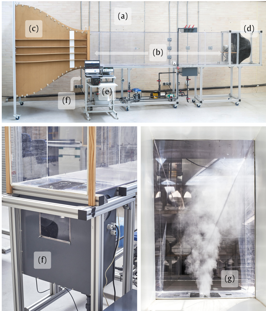
Figure 1: Photographic view of the test rig: (a) subsonic wind tunnel, (b) test section, (c) nozzle, (d) diffuser, (e) data acquisition system, (f) ultrasonic mist generator and (g) structure of water mist stream.
