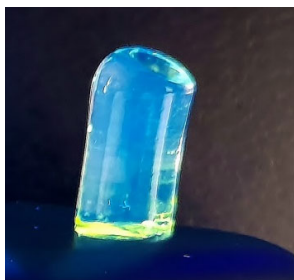
Figure S4. Digital image of ex situ F8BT@AETA hydrogel taken under irradiation with UV light (365 nm) after three days of preparation.
