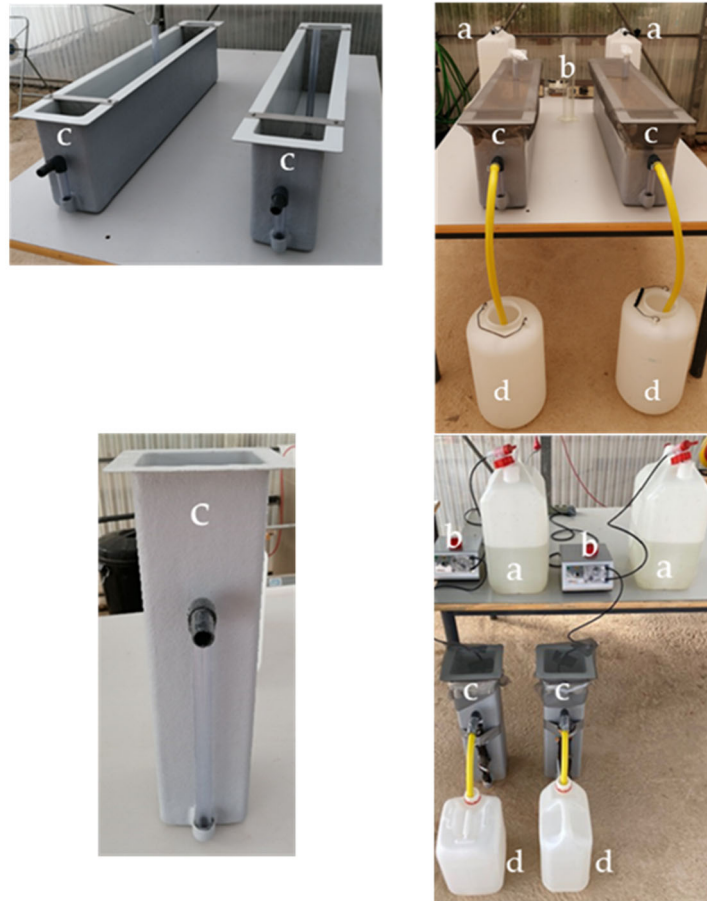
Figure 2. Bioreactors diagrams. At the top: anaerobic bioreactor with subsurface water and horizontal flow. At the bottom: anaerobic bioreactor with subsurface water and vertical flow. (a) irrigation water in polyethylene deposits; (b) peristaltic pump; (c) biofilter; (d) effluent recovered in polyethylene deposits.
