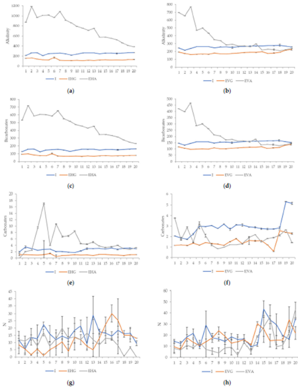
Figure 4. Alkalinity, bicarbonates, carbonates and N results of horizontal and vertical water flow bioreactors. (a) Weekly alkalinity concentration ( \text{mg L}^{-1} ) of horizontal water flow bioreactors. (b) Weekly alkalinity concentration ( \text{mg L}^{-1} ) of vertical water flow bioreactors. (c) Weekly bicarbonates concentration ( \text{mg L}^{-1} ) of horizontal water flow bioreactors. (d) Weekly bicarbonates concentration ( \text{mg L}^{-1} ) of vertical water flow bioreactors. (e) Weekly carbonates concentration ( \text{mg L}^{-1} ) of horizontal water flow bioreactors. (f) Weekly carbonates concentration ( \text{mg L}^{-1} ) of vertical water flow bioreactors. (g) Weekly N concentration ( \text{mg L}^{-1} ) of horizontal water flow bioreactors. (h) Weekly N concentration ( \text{mg L}^{-1} ) of vertical water flow bioreactors.
