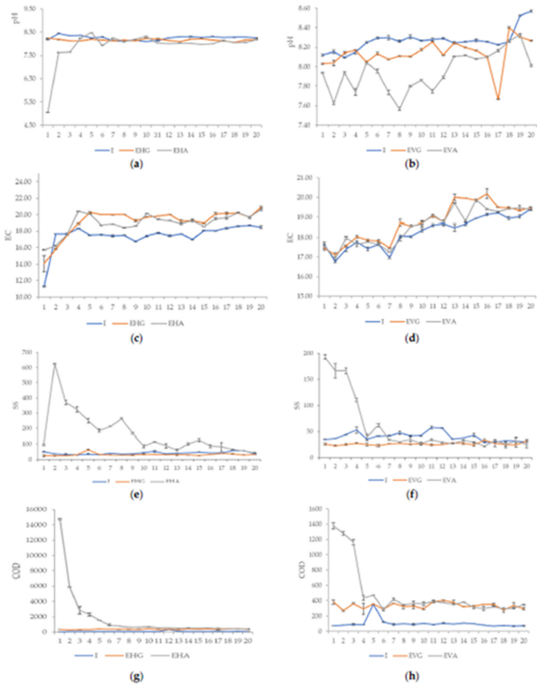
Figure 3. pH, EC, SS and COD results of horizontal and vertical water flow bioreactors. (a) Weekly pH (units) of horizontal water flow bioreactors. (b) Weekly pH (units) of vertical water flow bioreactors. (c) Weekly EC (mS cm -1 ) of horizontal water flow bioreactors. (d) Weekly EC (mS cm -1 ) of vertical water flow bioreactors. (e) Weekly SS concentration (mg L -1 ) of horizontal water flow bioreactors. (f) Weekly SS concentration (mg L -1 ) of vertical water flow bioreactors. (g) Weekly COD concentration (mg L -1 ) of horizontal water flow bioreactors. (h) Weekly COD concentration (mg L -1 ) of vertical water flow bioreactors.
