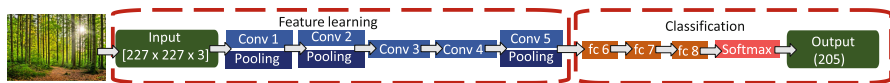
Fig. 1. Architecture of the Places CNN [12]. This network was created to address a scene recognition task among 205 types.
