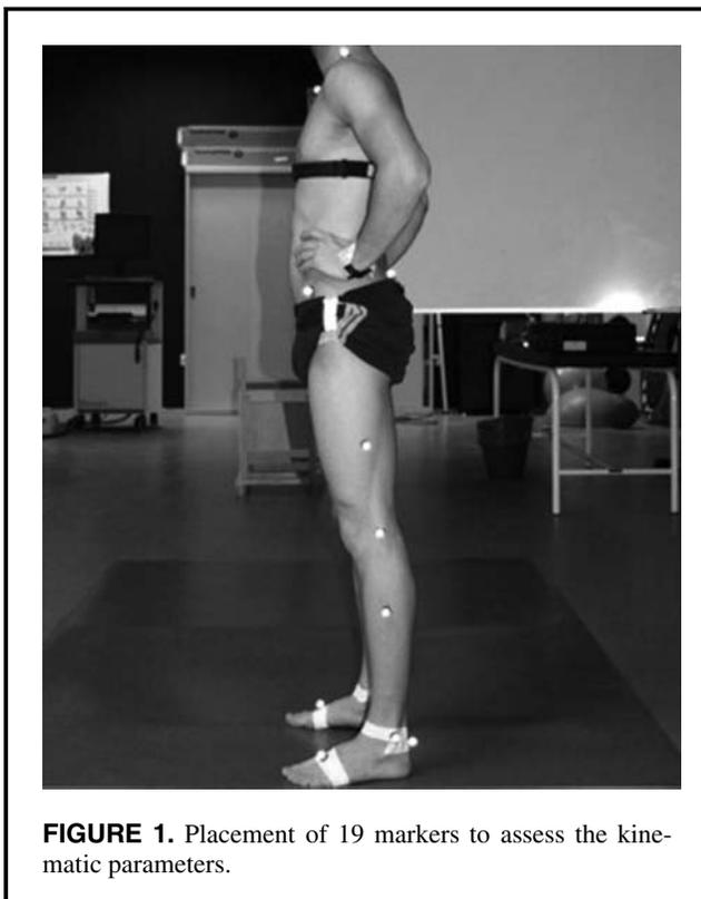
**FIGURE 1.** Placement of 19 markers to assess the kinematic parameters.
