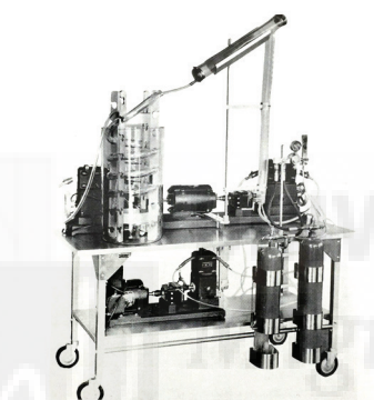
FIGURE 1. The total cardiopulmonary bypass apparatus. Venous blood drains by gravity to the venous reservoir (lower shell, center right), from which it is pumped to meet an oxygen stream in the vertical mixing tube. The oxygenated blood is then debubbled in the obliquely placed chamber. From there the blood flows into a helical reservoir in the lower water bath. This helical reservoir serves several purposes: (1) It completely oxygenates the oxygenated blood from any small bubbles or air gas that may have passed from the debubbling tube. The air gas has a lower density than water, and is thus carried upward. (2) Normal body temperatures are maintained by the helical coil in a constant upper portion of blood vessel as a level indicator to balance the input and output of the oxygenator. (3) The coil serves as a reservoir for the oxygenated blood until flow to the heart. (4) The blood is returned to the patient by the "arterial" pump head (center left, upper shell). The centrifugal pump, reservoir, and pump are shown on the lower shell. The blood from this source is also pumped in the vertical mixing tube. The double mixing tube and debubbling system is used for perfusions requiring larger quantities of blood (2000 cc. of blood per minute and up).
