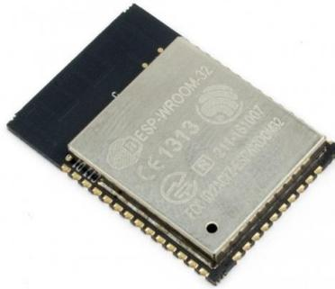
*Figura 43 – Módulo ESP32-WROOM-32 [45]*
