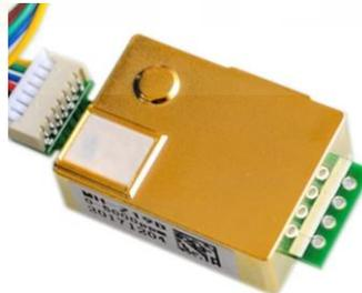
Figura 35 – Sensor CO<sub>2</sub> – MHZ-19B [37]
