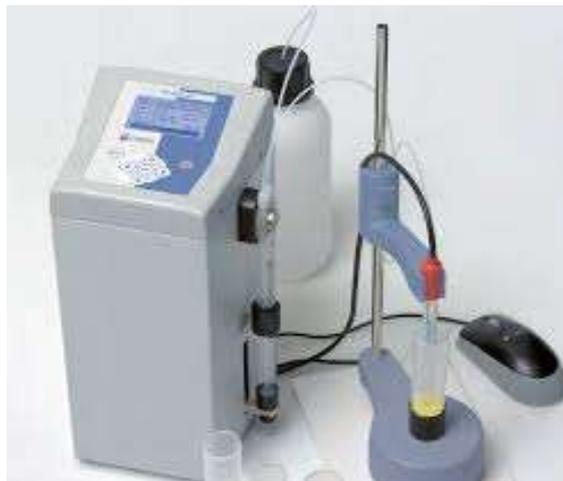
Figura 8: Titrador CRISON PH-MATIC 23 ([www.crisoninstrument.com](http://www.crisoninstrument.com))
