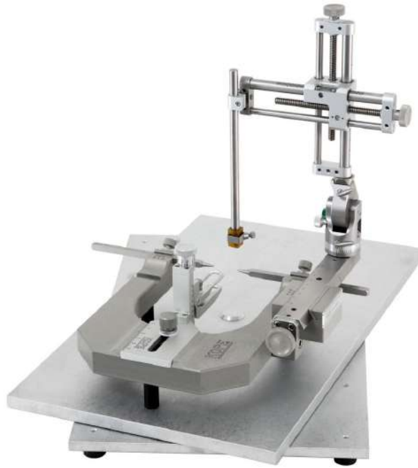
Fig. 5 Kopf Dual Small Animal Stereotaxic Instrument, Model 902 (44).
