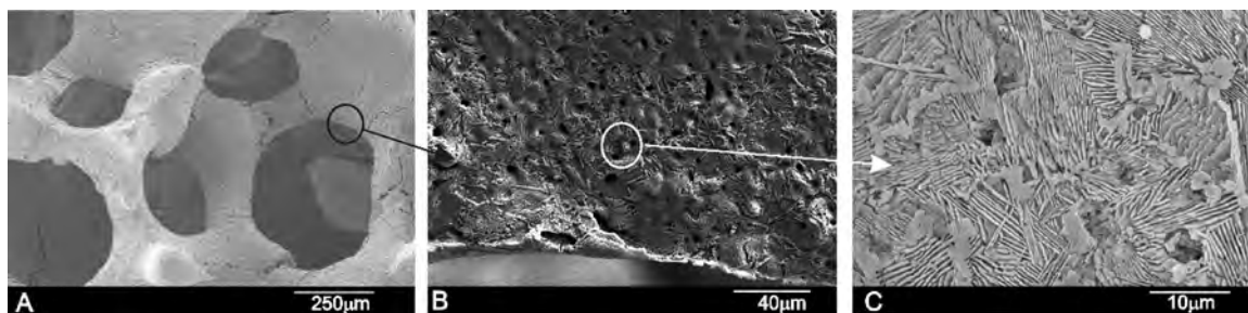
Fig. 1. SEM micrographs of the (A) ceramic scaffold; (B) detail of the strut; (C) irregular lamellar microstructure.
