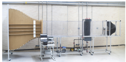
Fig. 3. Overall view of the subsonic wind tunnel and position of the evaporative pad tested.
