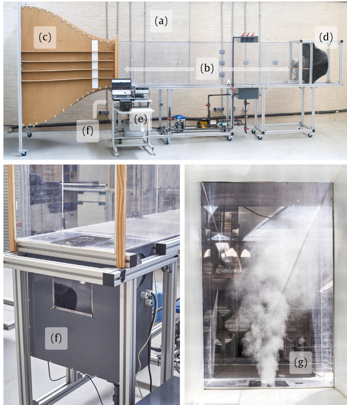
Fig. 1. Photographic view of the test rig: (a) subsonic wind tunnel, (b) test section, (c) nozzle, (d) diffuser, (e) data acquisition system, (f) ultrasonic mist generator and (g) structure of water mist stream.
