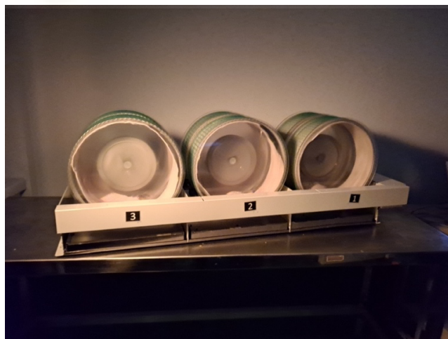
Figura 3. Forced Exercise / Walking Wheel System for Rats de la empresa Lafayette Neuroscience. Modelo 80805. Elaboración propia
