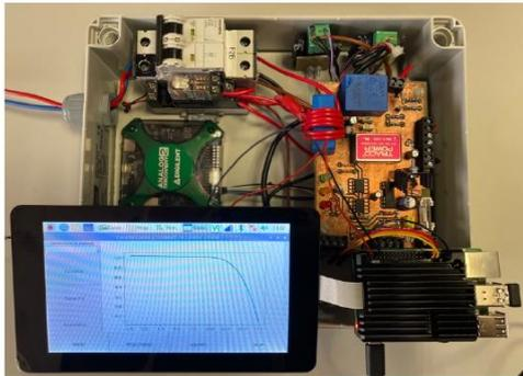
Figure 5 IV curve tracer system (not assembled)
