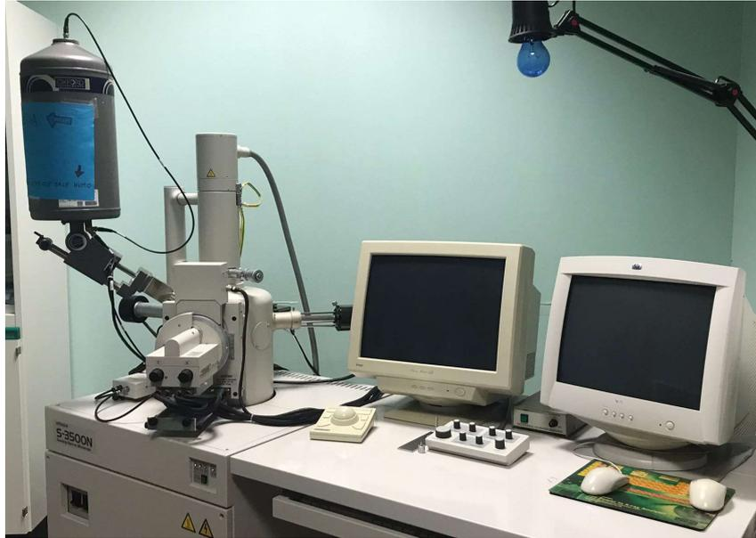
**Figura 14.** MEB SEM-HITACHI S-3500N y MED-RX OXFORD LINK ANALITICAL.
