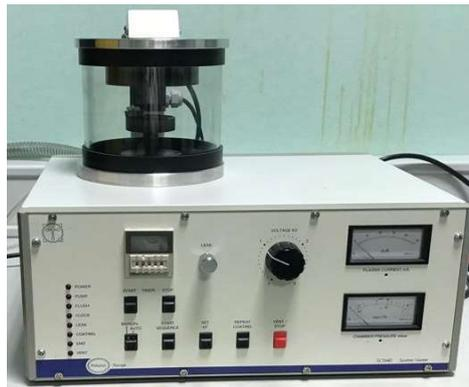
**Figura 13.** Recubridor Polarion (modelo SC7640, Quorum Technologies).
