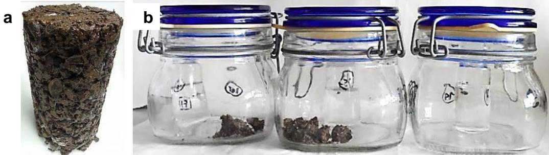
**Figure 9 - a:** Aspect of the mixture after being taken from the reactor; **b:** hermetic jars with sample and CO<sub>2</sub> traps.
