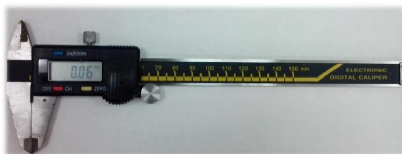
FIGURA 10. CALIBRE DIGITAL MITUTOYO 150 MM
