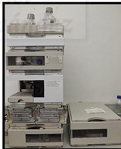
Figura 22. HPLC Hewlett Packard HP 1100.
