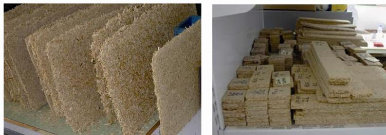
**Fig 2. (left)** Finished particleboards during conditioning at 20 °C and 65% relative humidity;
